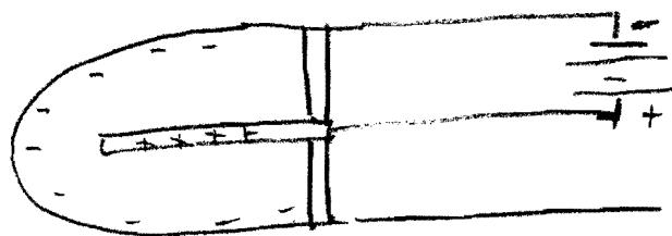
When radiation strikes the gas molecules within the chamber, the molecules become ionized:
