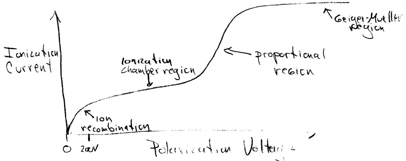
At 0 Volts, there is no current since the electrodes don't attract the electrons. The ion pairs simply re-combine.
